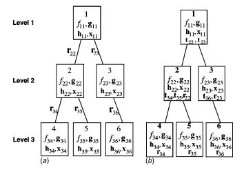
Fig. 1 (a) Hierarchical problem structure and variable allocation for ATC; (b) variable allocation for ATC after introducing target copies
