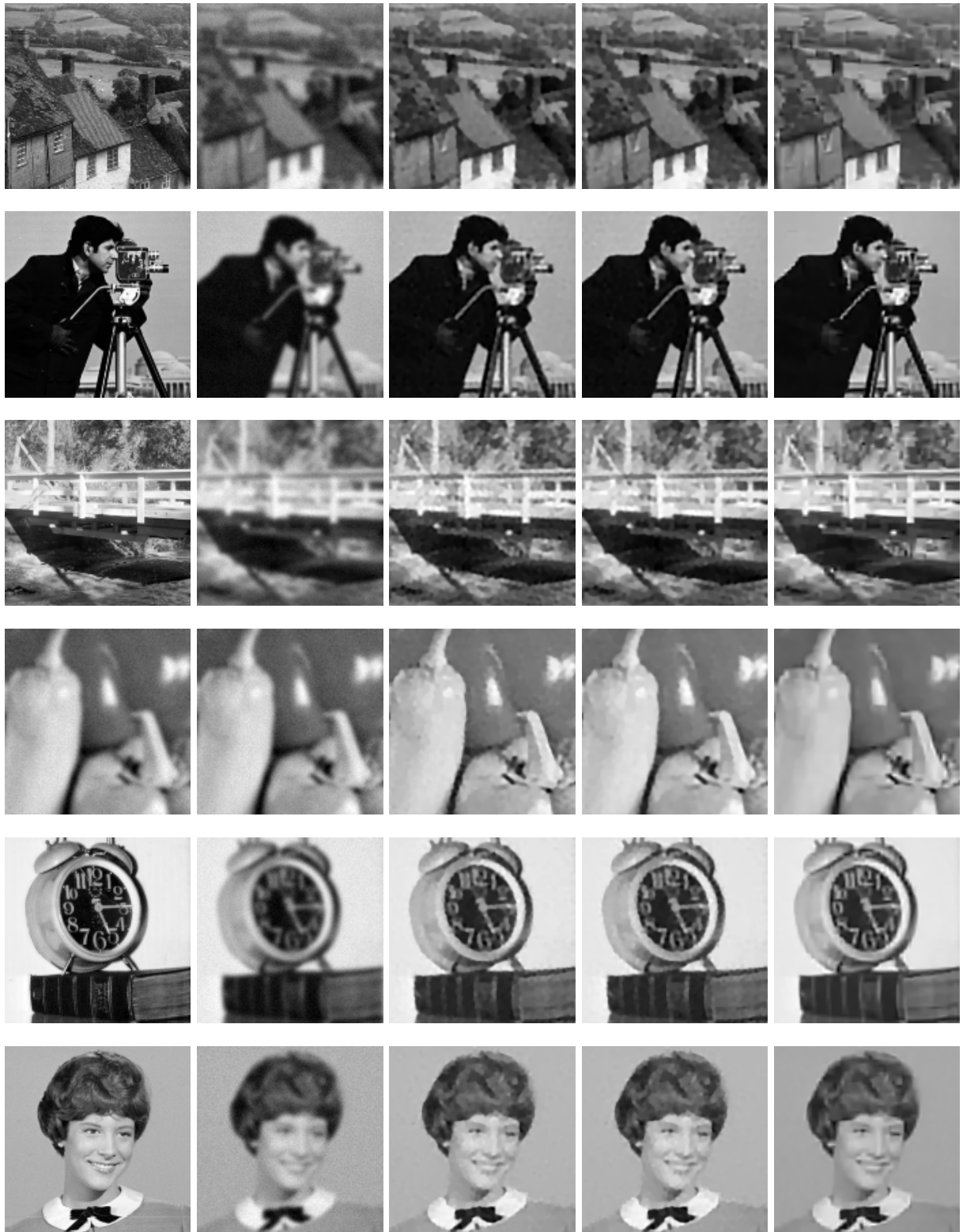
FIGURE 3. Zoom-in to the texture part of “downhill”, “cameraman”, “bridge”, “pepper”, “clock”, and “portrait I”. Image from left to right are: original image, observed image, results of the balanced approach, results of the analysis based approach and results of the PD method.
